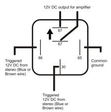
For Aquatic AV stereos, position 86 can be connected to either the blue remote wire in the harness or the brown 12V trigger on the rear of the unit. There differences are below:
